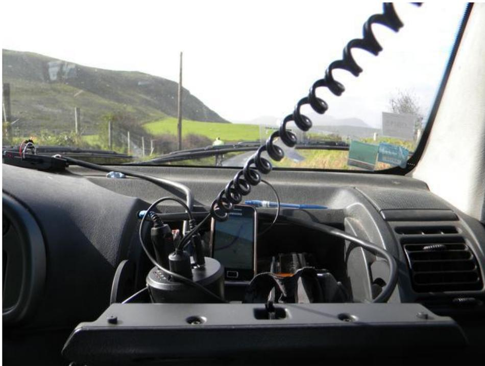
The electronic gear in the following car, featuring the câble for the roof orange light, the BlackBlox GPS device giving our position to race headquarters, and an Android
